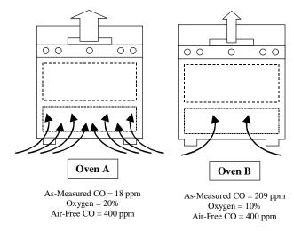
10 percent, the percentage of  $O_2$  for a natural gas or propane oven is much higher, normally within a range of 14 to 20 percent. This Oven A, the as-measured CO level is 18 ppm; safe by most higher range of  $O_2$ (excess air) in the combustion gases leads to *lower* as-measured readings.
