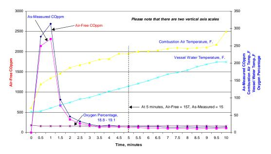
The graph below is for burner 2, test type B. Please note that there are two vertical axis scales.
