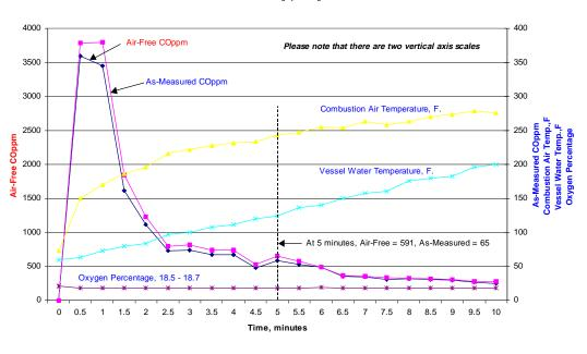
The graph below is for burner 1, test type B. Please note that there are two vertical axis scales.
