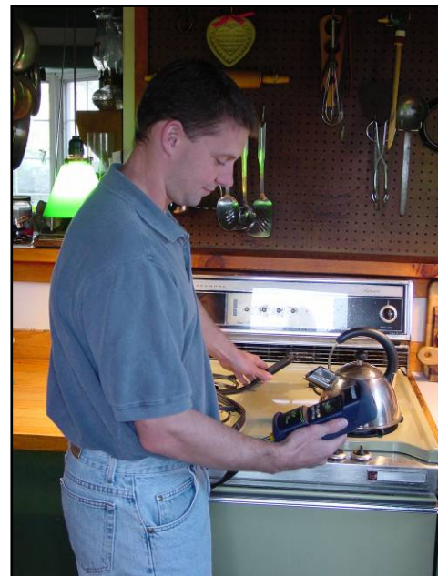
Testing gas oven for CO emission level
