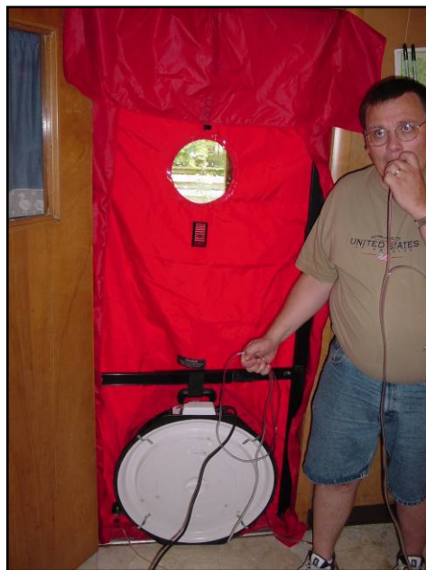
Setting up the blower door for a depressurization test
