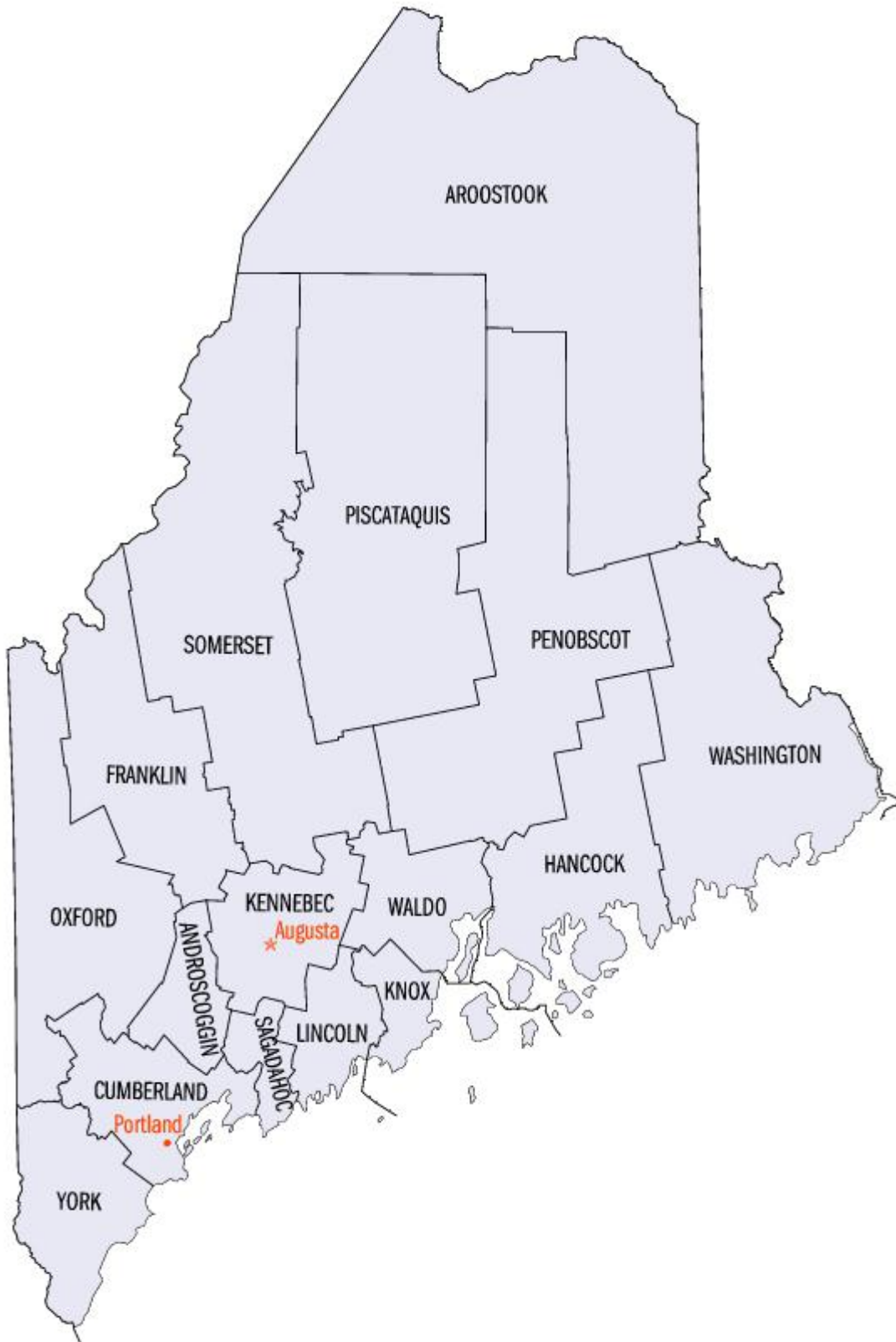
Figure 2. County map of Maine. The Maine Model Building Energy Code divides the state into two zones. One zone is Aroostook county and the other zone includes all other counties.
